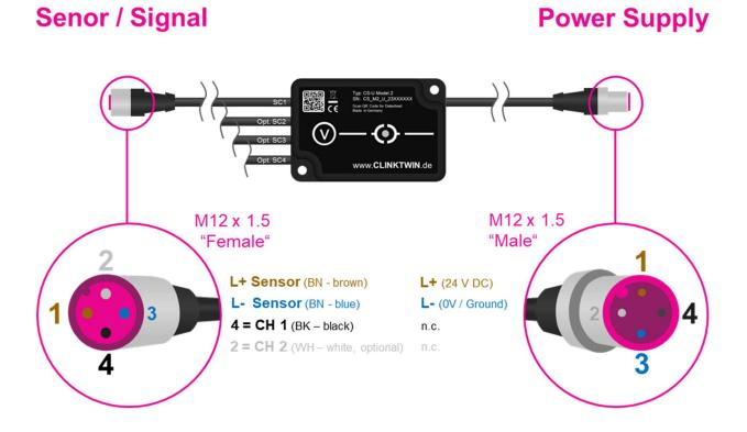
The Sensor Connection of all available **CLINKTWIN** Satellites is realized by using M12 x 1.5 Sensor Socket too ("Female", picture below left hand). Further connection Details as PIN assignment 1 to 4, colouring of cables as well as Plug assignment the can be taken from the illustration as well as from the List below:
