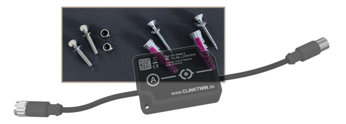
The **CLINKTWIN** CH Hub housing is designed to fit to standardized DIN rail. Rail and Hub, clean environments assumed, can be mounted by fixing the DIN rail with 2 x SPAX Screw (+Dowel) direct to any building wall, or, by use of the further available metric M4 Screws, to any other underground.
