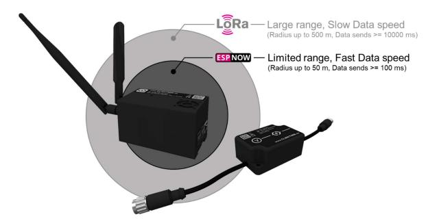
Even the option to cover a wide range by using fast data speed is possible, only ends up in the need for additional Hub's.
